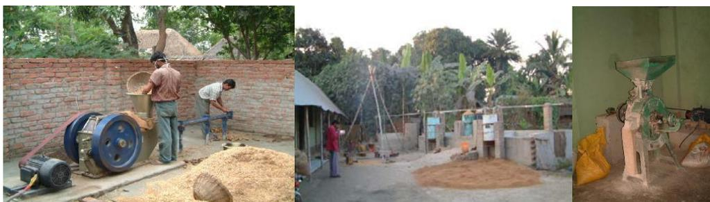
Right at the start, villagers identified irrigation water as their most needed input. DESI Power and BOVS worked out a solution which was based on selling water rather than electricity: under ground power lines and pumps were installed in the fields and a channel-based supply system was set up. The irrigation pumps run for 5-6 months in a year for 10-12 hours daily. About 200 acres of land are under cultivation in which different types of crops such as, paddy, wheat, maize, dhaincha, jute,
